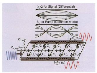
Distributed parametric resonator for frequency division. When a pump is applied (changing capacitance), the ambient noise grows through parametric amplification by traveling back and forth between two reflective ends. Finally, it generates stable output at half of the pump frequency. In this way, the energy from the signal is transferred to its half frequency component without any static power consumption. This results in very low phase noise operation.
